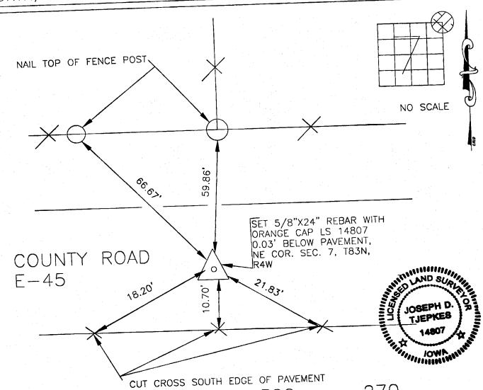
PREVIOUSLY RECORDED IN BOOK 302, PAGE MONUMENT DESCRIPTION AND HOW ESTABLISHED FOUND CROSS IN PAVEMENT PER CORNER TIES IN BOOK AND PAGE INDICATED ABOVE. THE BRASS PLUG SHOWN IN TIES WAS GONE. DRILLED HOLE AND SET 5/8"X24" REBAR WITH ORANGE CAP LS 14807 0.03' BELOW PAVEMENT AND ESTABLISHED NEW TIES.
