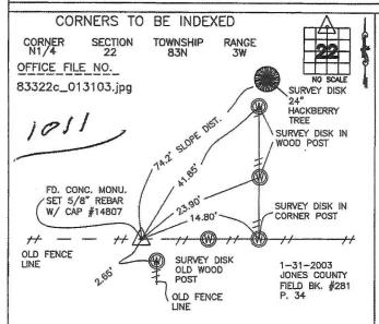
PREVIOUSLY RECORDED IN BOOK NA , PAGE NA MONUMENT DESCRIPTION AND HOW ESTABLISHED FROM 1936 TIES RECORDED AT JONES COUNTY ENGINEERS OFFICE FD. CONCRETE MONUMENT UNDER FENCE LINE. SET 5/8"X48" REBAR W/ CAP #14807 ON EAST SIDE OF MONU. TOP OF REBAR 6" ABOVE GROUND LEVEL SET SMALL JONES COUNTY SIGN ALONG SIDE OF MONU, N1/4 SECTION 22 TB3N R3W. REFERENCE TIES AS INDICATED.
