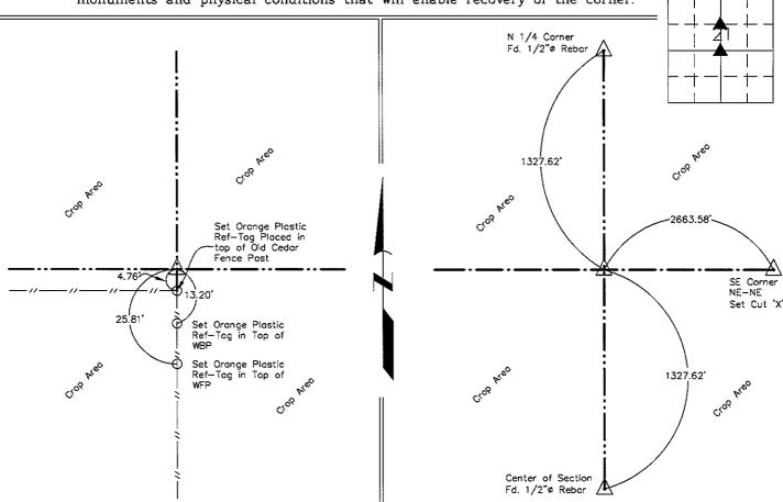
(1) CTR OF SECTION of Sec. 21-T85N-R3W Set 1/2" Rebar w/ Aluminum Cap LS No. 7060
